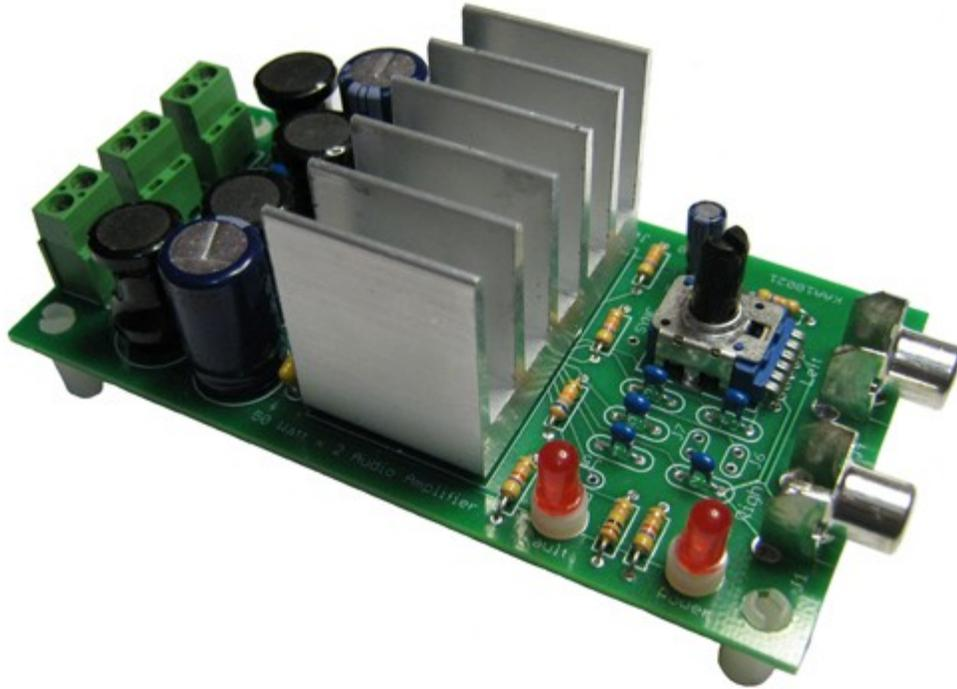
This amplifier kit uses Texas Instruments TPA3116D2 stereo audio amplifier IC for driving speakers up to 50 watts @ 4 ohm per channel in stereo mode and 100 watts @ 2 ohm in mono mode. It's efficient Class-D operation produces very little heat and with the oversized heat sink will only get slightly warm when cranking it up. Fault LED on board for indicating a Over-temp, DC detect or Open speaker / connections. The amplifier operates on 5 to 26 Volts DC.
